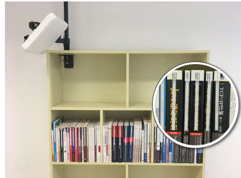
Fig. 6. The white antenna is placed at a 45^\circ angle to the ground to ensure it can cover as much region as possible, because of its fan-shaped radiation regions.
